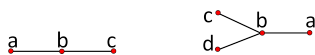
Figure 11: Edge-collapsed graph for two different cells. The nodes in each graph represent distinct faces of the cell. The labels for the nodes with assigned integer values represent the layer number of the face. The graph on the left is linear with three nodes and guarantees an embedding, whereas the graph on the right does not have a linear spanning subtree and does not guarantee an embedding
