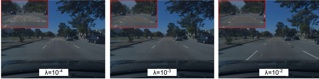
Figure 7: Driver’s view at 2.5 sec (average driver reaction time to road hazards [57]) before our attack succeeds under different stealthiness levels in local road scenarios. Inset figures are the zoomed-in views of the malicious road patches. Larger images are in our extended version [38].
