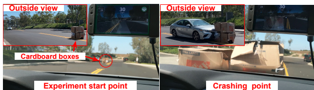
Figure 14: Safety impact evaluation for our attack on a Toyota 2019 Camry with OpenPilot engaged. Even with other driver assistance features such as Automatic Emergency Braking (AEB), our attack still causes collisions in all the 10 trials.
