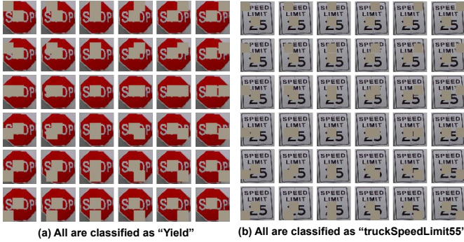
Fig. 16: Mis-certified examples of two-round masked images. (a) For the stop sign, all images are classified as a “Yield” sign in the 4%-pixel patch scenario. (b) For the speed limit sign, all images are classified as a “truckSpeedLimit55” sign in the 2%-pixel patch scenario.
