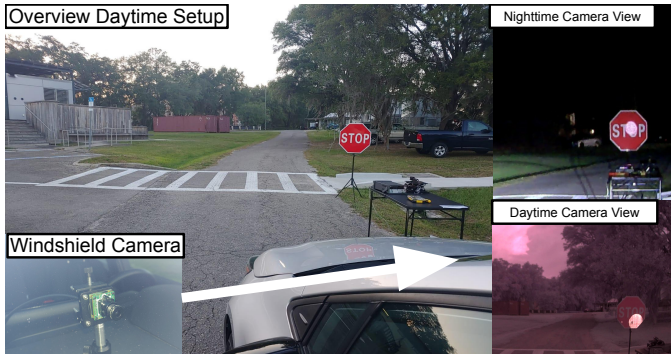
Fig. 13: Overview of the outdoor experimental scenarios. The setup is used in the daytime (left). The camera view during the attack is at nighttime (Right-top) and daytime (Right-bottom).
