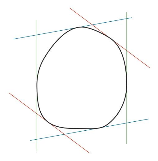
Diam = max distance between parallel tangents Width = min distance between parallel tangents
