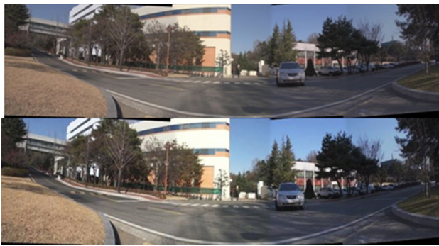
Fig. 13 Generated Office building panoramas when: (upper) least suitable reference I_1 and (lower) most suitable reference I_4 is selected by proposed scheme
