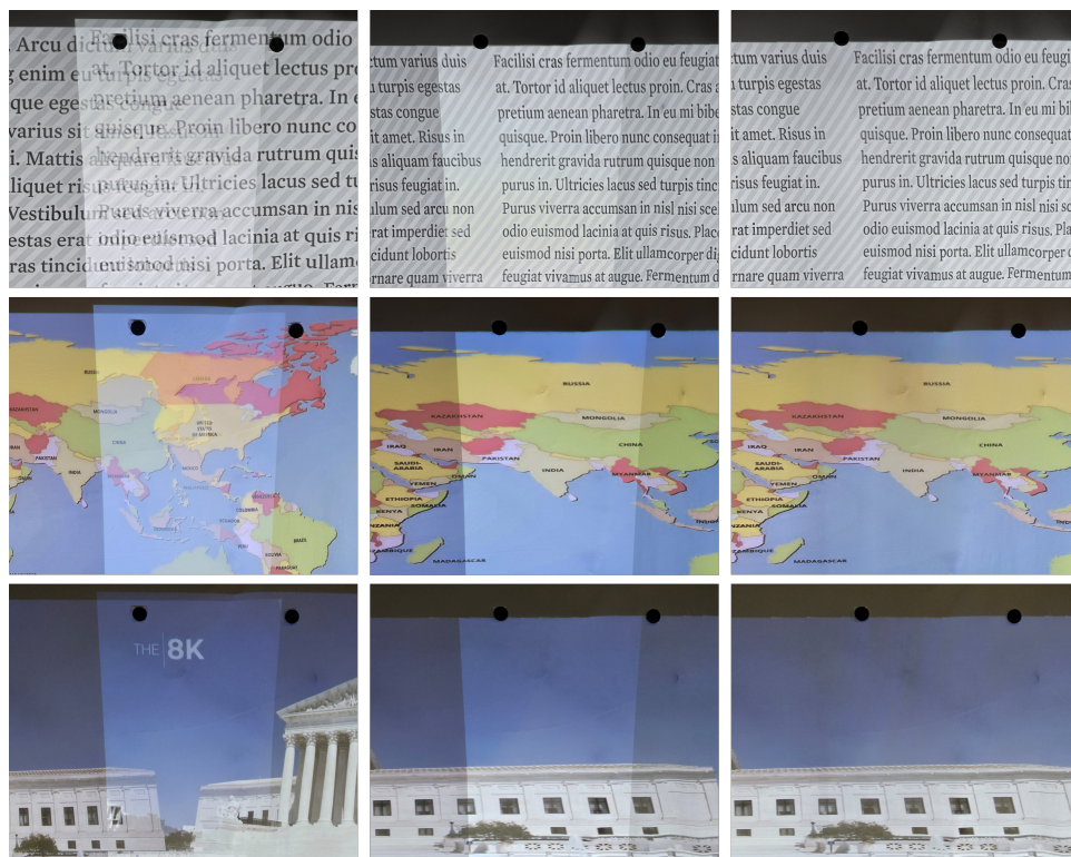
Figure 8: Results of our calibration, rendering and display method. Left column : No calibration. Middle column : Calibrated result without blending. Note the accuracy of our registration. Right column : Our final blended result.
