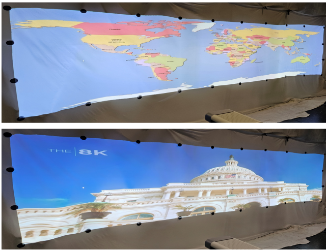
Figure 7: The final multi-projector display on a moving, deformable surface.
