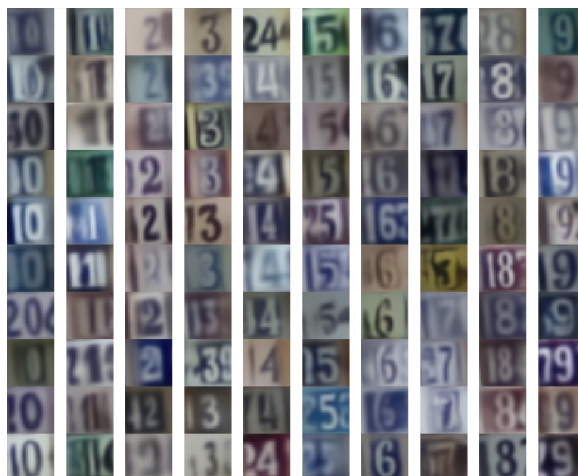
Figure 13: Class-conditional samples of the 10 possible digit classes in the SVHN dataset. The generative model was trained on the fully labeled SVHN dataset with prediction and consistency constraints. Samples were chosen via rejection sampling in the latent space with a threshold of 95% confidence in the target class.
