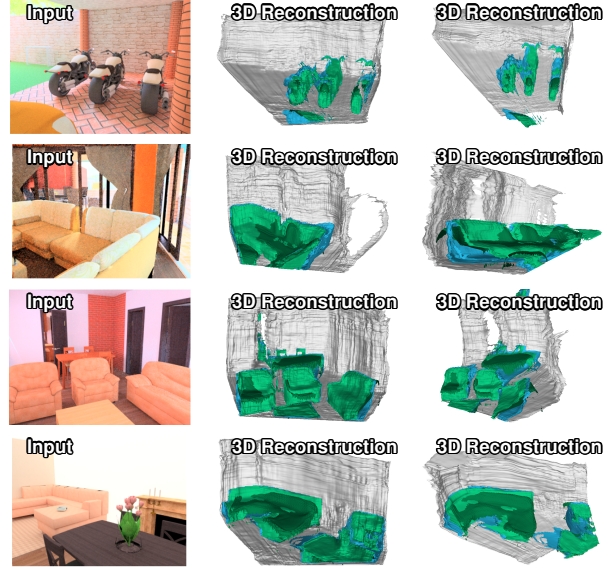
Figure 5: Single image scene reconstruction via multi-layer depth maps. Estimates of the front (green) and back (cyan) surfaces of objects, as seen from the input view, are complemented by heights estimated by a virtual overhead camera (dark green) via our epipolar feature transform. Room envelope estimates are rendered in gray.
