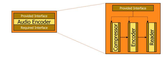
Compressor IS-COMPONENT-OF Audio Encoder Encoder IS-COMPONENT-OF Audio Encoder Reader IS-COMPONENT-OF Audio Encoder Compressor, Encoder, and Reader IMPLEMENT Audio Encoder Audio Encoder IS-COMPOSED-OF Compressor, Encoder, and Reader
